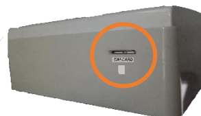
Fig. 6. Sim Card Slot of the Device
