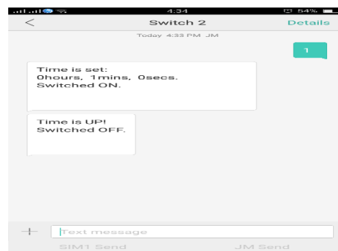
Fig. 9. Time is up SMS message of the device
